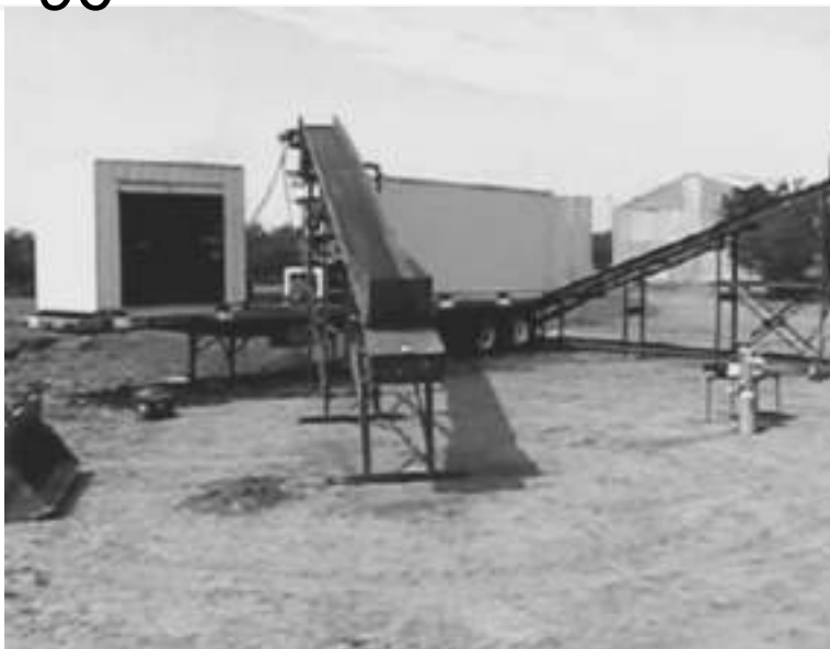
Figure 14. Portable VEG-based ex-site PFAS-contaminated soil remediation unit (Endpoint Consulting,
